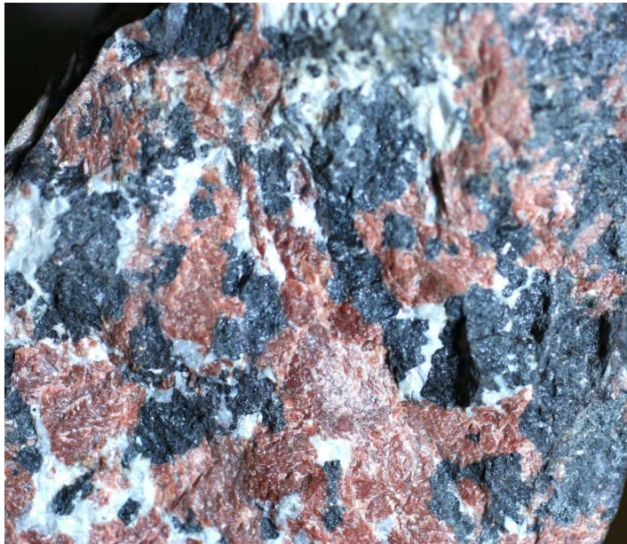
Figure 13. Typical Sterling Hill ore sample, consisting of willemite (pinkish brown), franklinite (black), and calcite (white), from the 1400 level, Sterling mine. Sample is 10 cm across. (Carnein specimen and photo)
