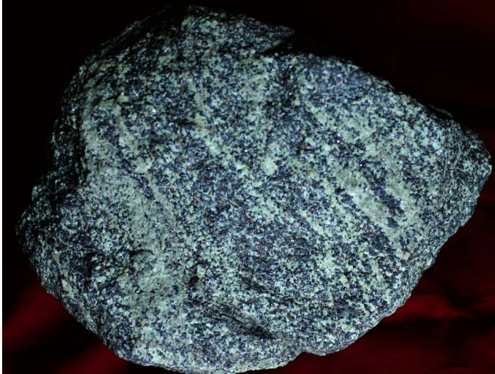
Figure 12. Typical Franklin gneissic ore, consisting of willemite (gray-green), franklinite (black), and minor zincite (red). Sample is 23 cm across. (Carnein specimen and photo)
