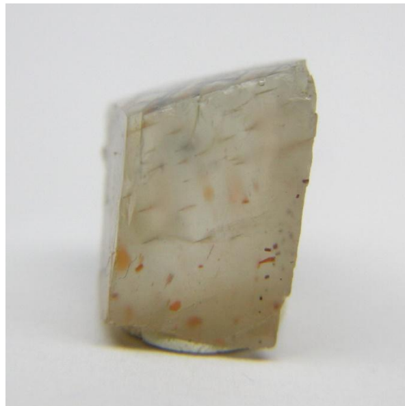
Figure 13. Side view of Figure 11, showing hematite flakes and very thin ilmenite blades in edge view. (Darren Arthur photo)
