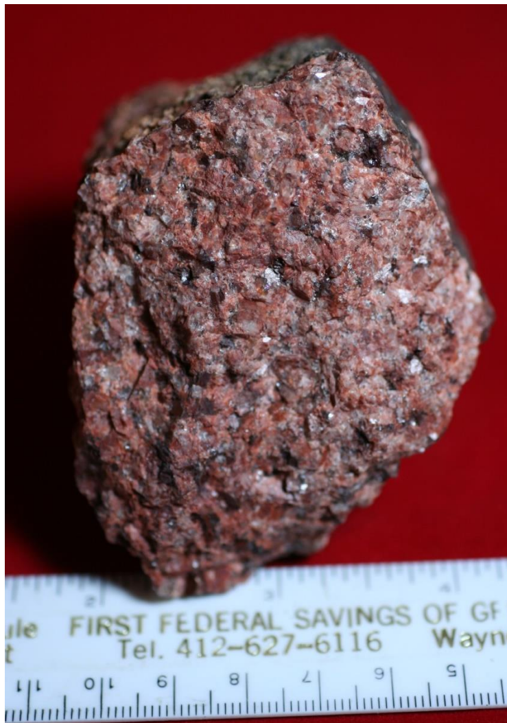
Figure 2. Coarse texture caused by slow cooling of magma beneath Earth's surface. Pikes Peak Granite. Minerals are quartz (pale gray), potassium feldspar (pinkish), and biotite (black). Plagioclase feldspar is also present. (Carnein photo and collection)
