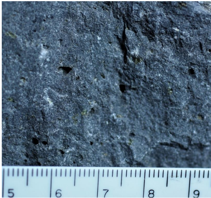
Figure 1. Volcanic rock (basalt), showing very fine grained texture due to rapid cooling from a melt. The rock consists mainly of plagioclase, pyroxene, and olivine. San Carlos Reservation, Arizona. (Carnein photo and collection)
