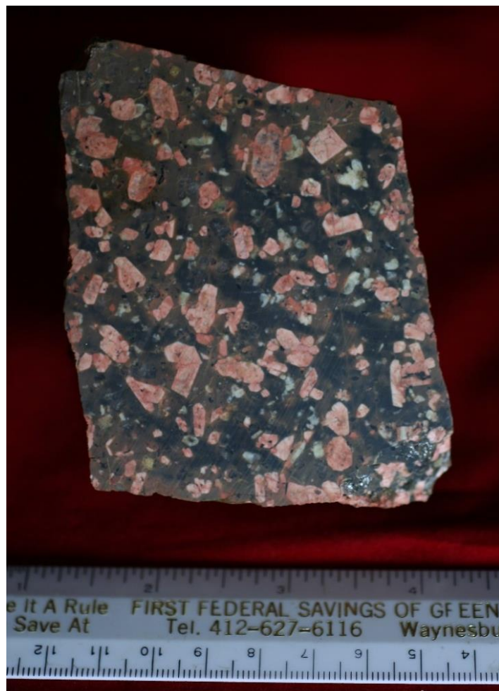
Figure 3. Porphyritic texture, caused by crystallization of magma under changing conditions. Pink and light gray crystals are potassium feldspar and plagioclase; groundmass is dark brown or gray. Vanda Porphyry, Wright Valley, Victoria Land, Antarctica. (Carnein photo and collection)
