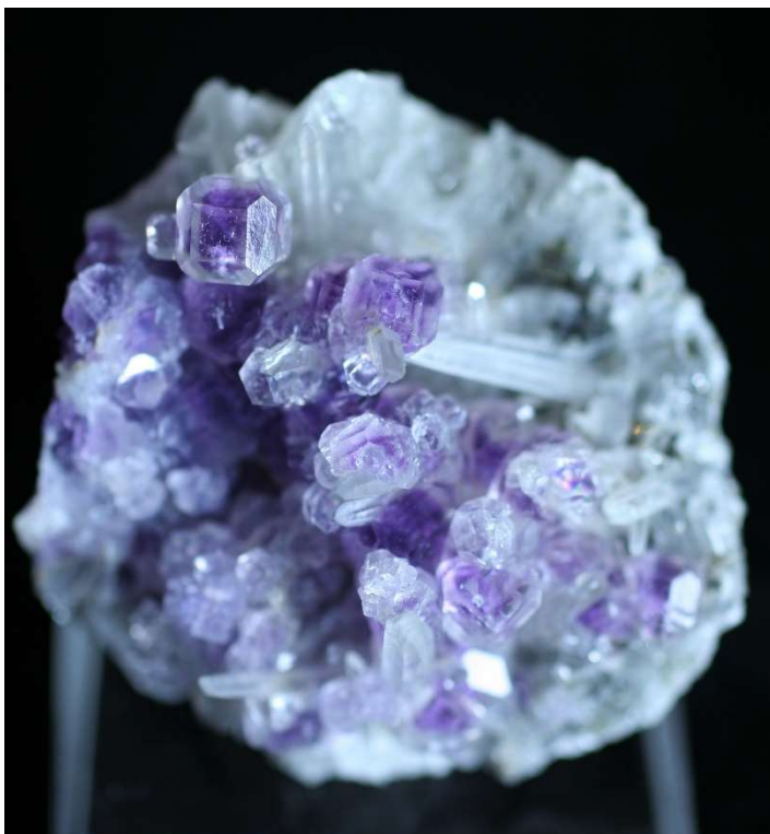
Figure 4. Fluorite with quartz and sphalerite from the Sweet Home mine. Note zoning and crystal habit of fluorite (cubes with dodecahedral edges).
