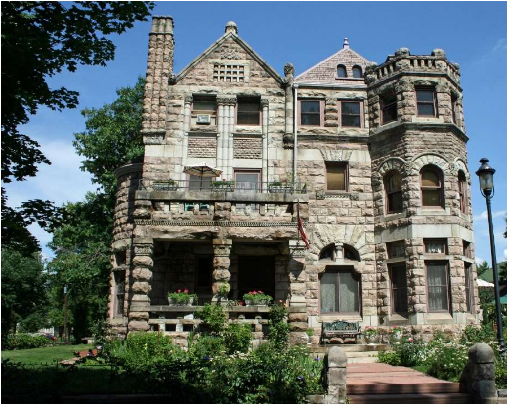
Figure 10. The Raymond House (Castle Marne) at 1572 Race Street, Denver is built largely of Castle Rock Rhyolite. Photo date July 2009 by Jeffrey Beall, permission to use through Creative Commons license.
