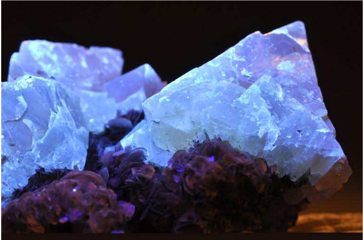
Figure 1. Scheelite crystals and muscovite mica showing fluorescence under ultraviolet radiation. Image courtesy of Commons Wikimedia: image released to public domain.
